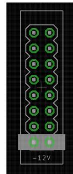
Line up the red stripe on the ribbon cable so that it matches the white stripe and/or -12 V indication on the board and plug in the connector.
